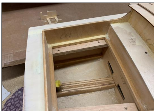
Modified rear access hatch showing lip for sealing strip, and attachment points for the securing bolts.
