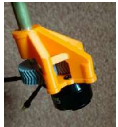
Figure 3 Designed and Printed Gearbox and Helical Gears on the Propshaft
