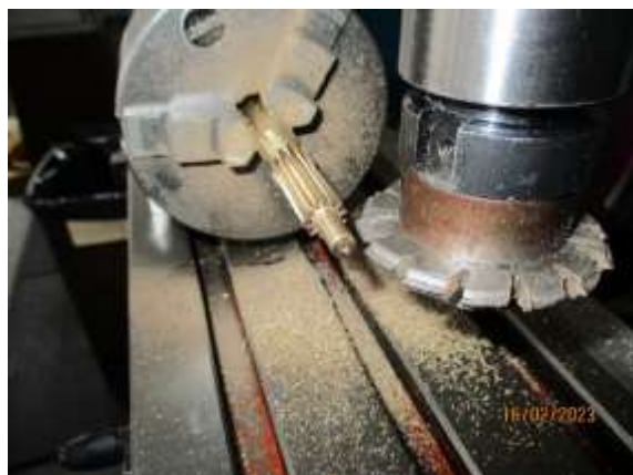
Cutting gears for oil pump
