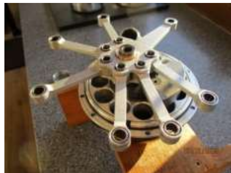
Figure 3 Con Rod Assembly with New Big End Bush
