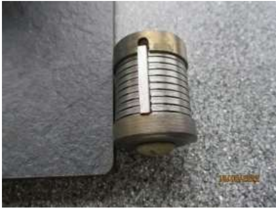
Jig for heat treating piston rings (held at red heat for 3 minutes and allowed to cool)
