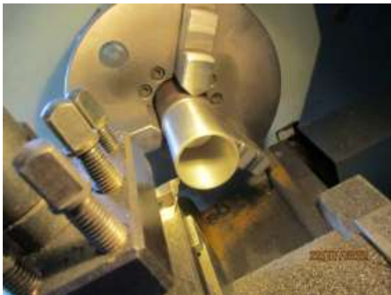
Turning mehanite tube to make piston rings
