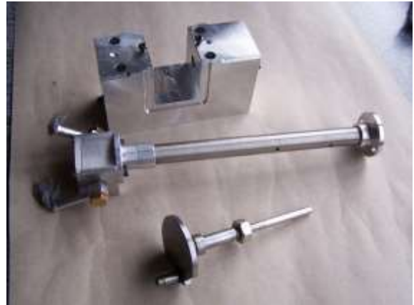
Rear housing containing crank shaft follower
