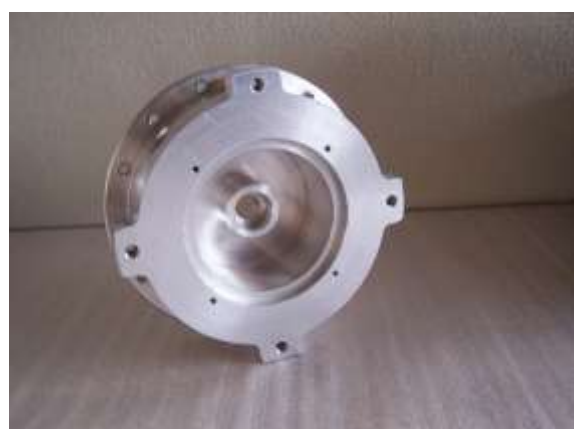
Rear housing machine from solid
