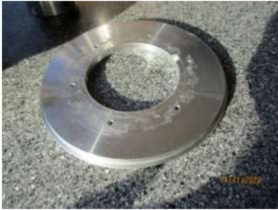
Cover plate for rear housing to form inlet manifold
