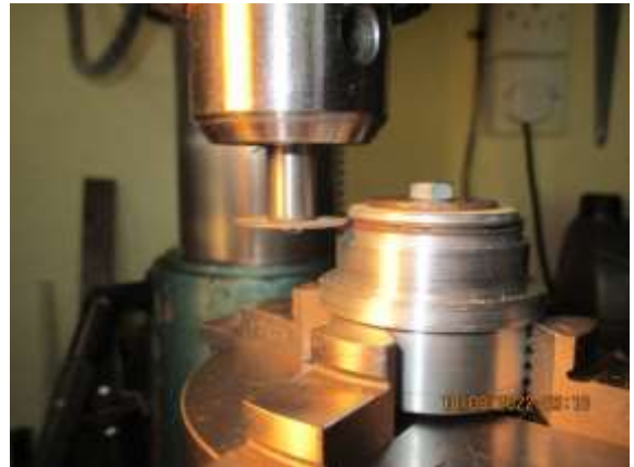
Machining slots for oil rings
