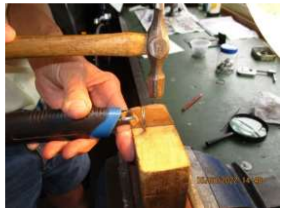
Splitting a piston ring, the ends of which will be trimmed up with a needle file to get the correct gap
