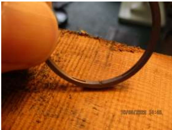
Using needle file to groove the ring ready for splitting
