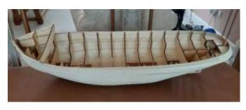
After sanding and filling a few gaps/blemishes with sawdust mixed with glue the inside and outside were covered and strengthened with fibreglass cloth and brushed using "Deluxe Materials Eze-Kote" laminating and finishing resin. More sanding and then the whole hull was sprayed with primer and below an approximate waterline 'Hull Red' paint.
